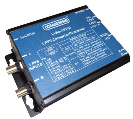
Multifunction interface for GNSS receiver 1 PPS signals
