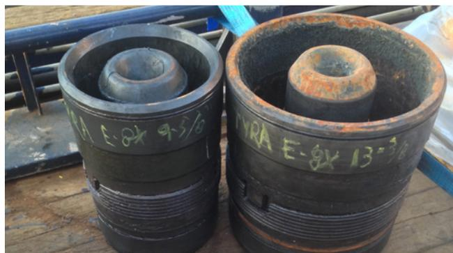
**Casing cutting and pulling:** With the project equipment spread already committed to using vessel deployed drill pipe tooling solutions, Motor-driven downhole casing cutters and spears were added to the suite of vessel deployed drill pipe tooling. The casing sizes for the internal cutting and pulling of casings included: 7 in, 9 5/8 in and 13 3/8 in to 800 ft below mudline.
