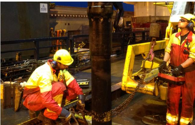
**Well Severance:** Oceaneering-supplied internal abrasive water jet and diamond wire cutting solutions were identified as the only appropriate options for final well severance. Explosive severance is still sometimes used in the industry; however, given the unknown consequences of peak pressure shock waves on the integrity of the remaining well barriers, let alone the damage caused to the marine flora and fauna, the use of explosives use, even as a backup, was not considered viable.
