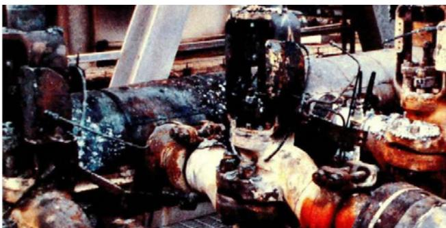
A gas leak caused a small but intense fire in a large petrochemical facility where Grayloc® connectors were used throughout the system. During the post-incident inspection, it was established that the connectors maintained their sealing integrity despite exposure to extremely high temperatures estimated at between 2,000°F and 3,000°F (1,090°C and 1,650°C).
