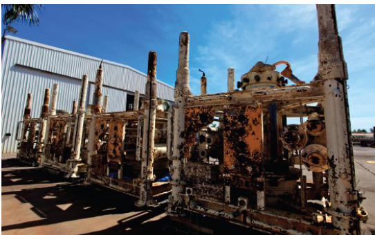
NORM Contaminated Subsea Trees
