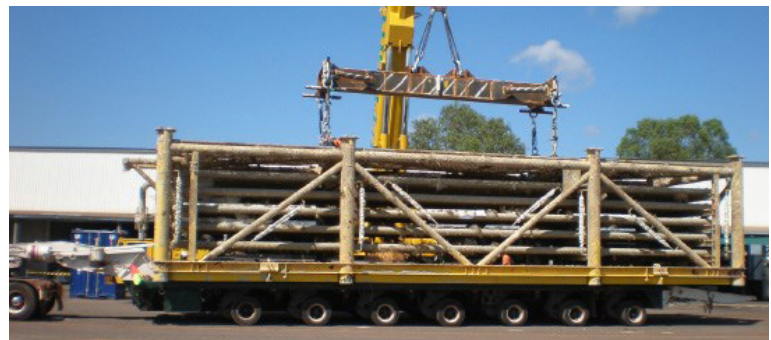
Contaminated Subsea Heat Exchanger
