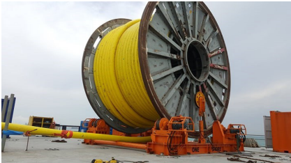
NORM Contaminated 300 Te Flexible Flowline
