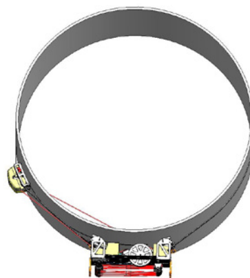
Cart moves around the object, while the diamond wire cuts
