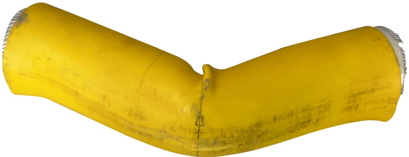
Completing a physical test on a length of umbilical can confirm the limit of axial compression or confirm if the design will take the predicted compression generated by the installation and operational analysis. The test can also determine the most likely failure mode and the extent of damage likely to occur.
