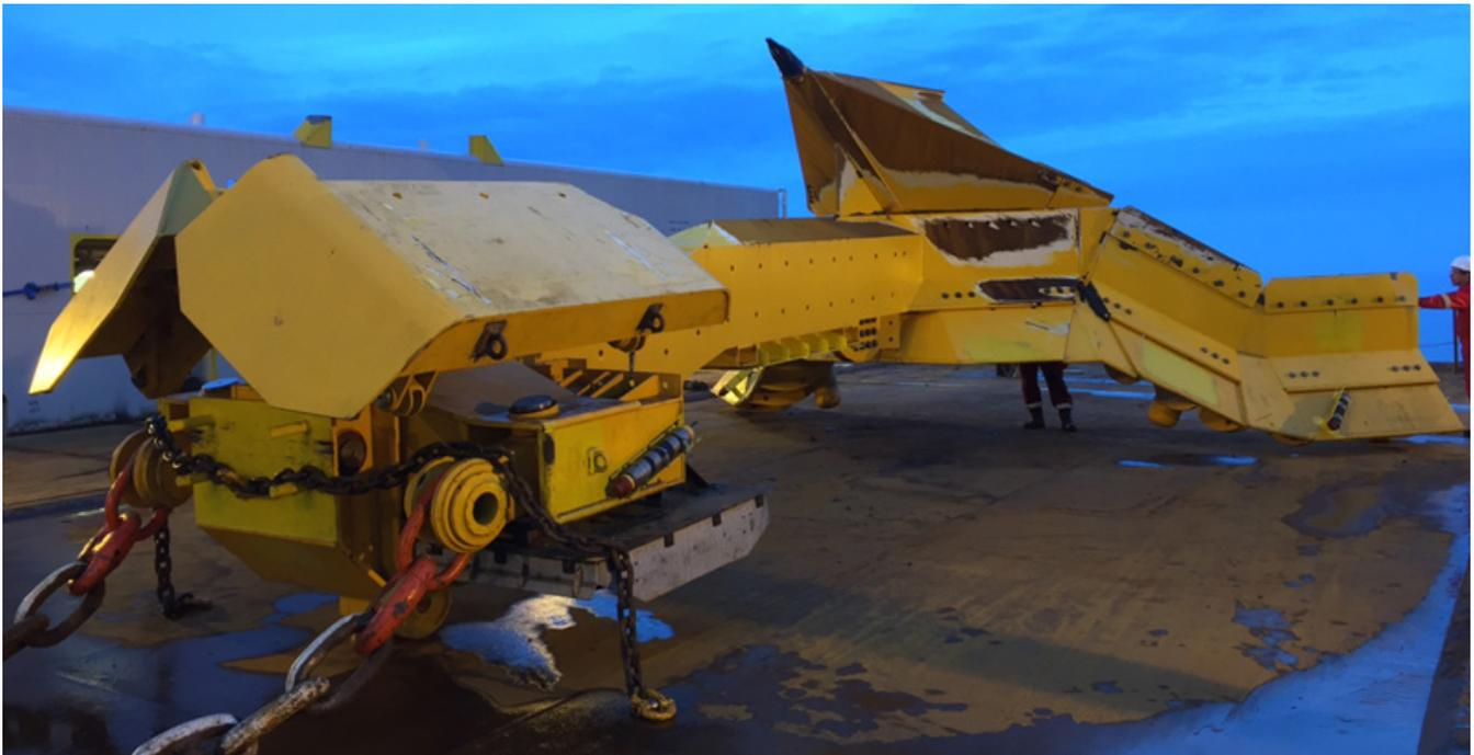
The SCAR Seabed System has been developed to deliver an all-in-one solution for route preparation prior to the burial of subsea cables, pipelines, and umbilicals.
