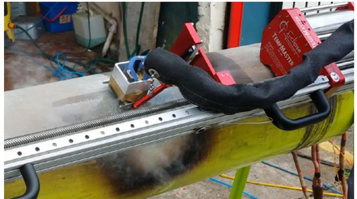
The system is specifically designed to operate at elevated temperatures and is used to evaluate the condition, particularly corrosion and weld inspections, of ferrous structures including storage tanks, pipelines, pressure vessels, and other critical equipment.
