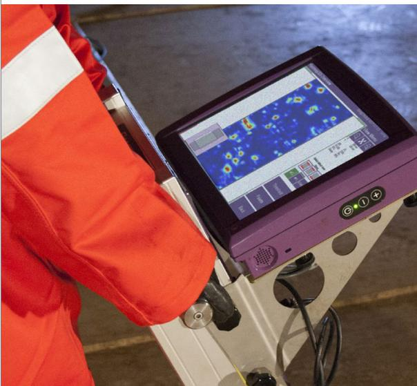
Oceanengineering offers advanced non-destructive tank inspection using the Silverwing Floormap3Di-R. The system is currently the fastest tank bottom inspection solution offered by Silverwing and provides scanning speeds up to 1 m/s—twice the speed of the previous model. The Floormap3Di-R increases inspection efficiency while improving accuracy and data quality.
