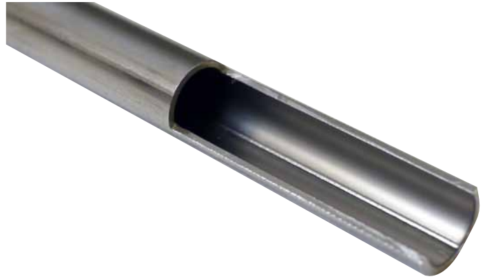
The tube has been machined to show the seam which is not visible on the outside of the tube.
