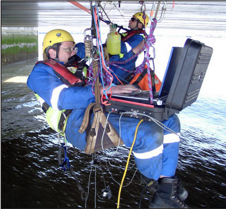
Oceaneering Rope Access technicians carrying out TOFD survey of the Thames Barrier, London.
