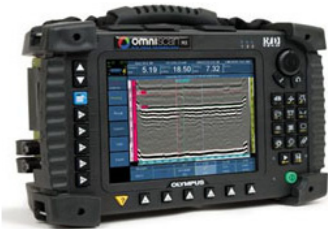
Omniscan unit used for ToFD inspection
