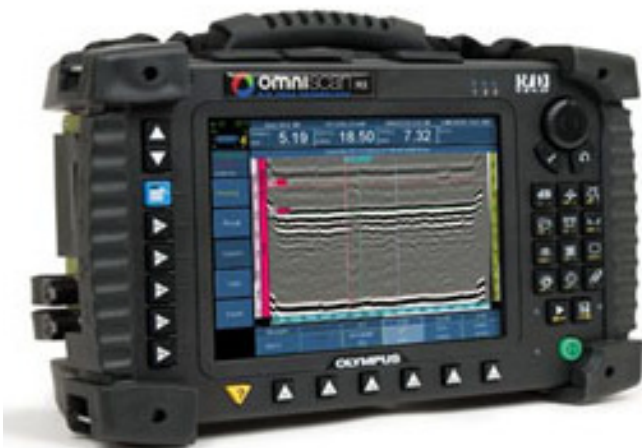
Omniscan unit used for ToFD inspection
