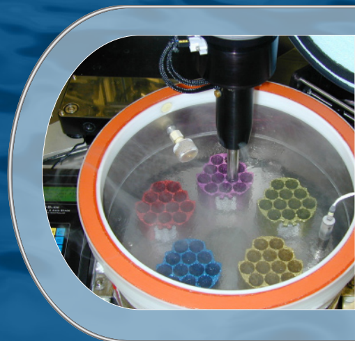
2 - Removing frozen crystals from storage
