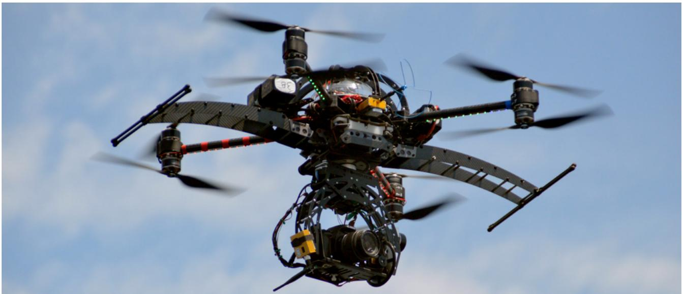
Oceanengineering uses UAS to inspect difficult-to-access locations both onshore and offshore. This agile and optimized solution often eliminates the need for rope access teams or other means of access and effectively minimizes risk and increases uptime for asset operators.
