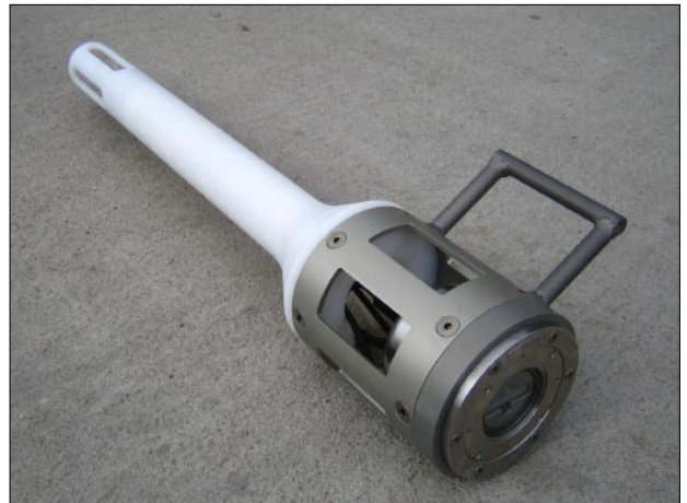
Subsea pH Meter Detects water pH value changes during the cementing phase.
